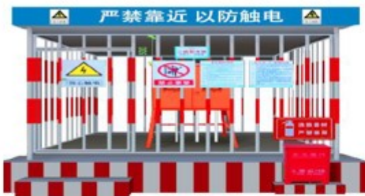
防砸、防雨挂牌上锁专人负责的二级箱 Anti - collision, anti - rain listing on the lock special person responsible for the secondary box
